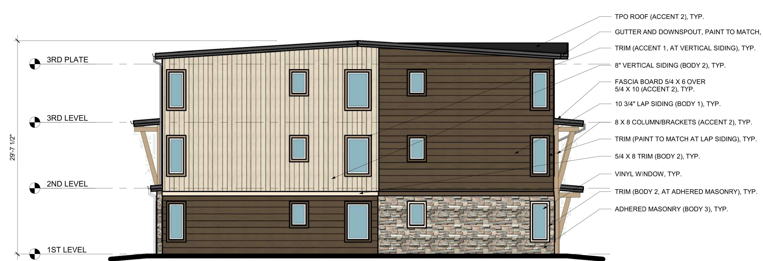
2 BUILDING 1 - WEST ELEVATION 1/8" = 1'-0"
