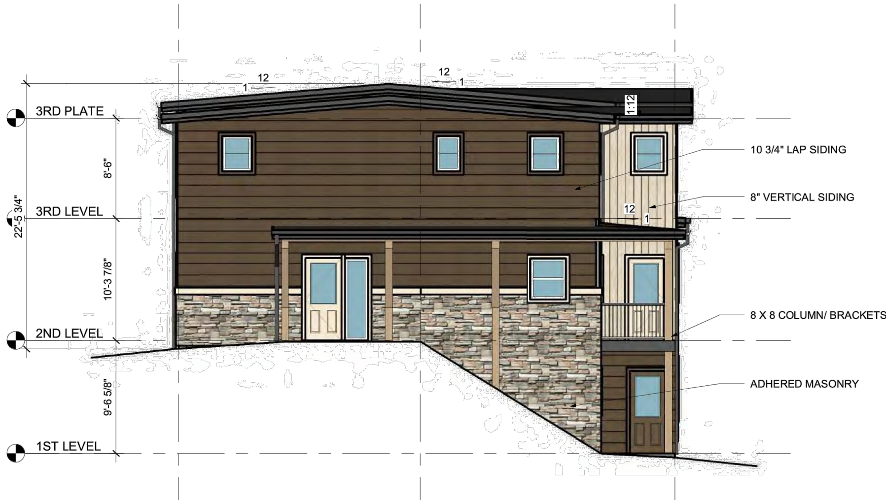
4 7-PLEX - LEFT SIDE ELEVATION 1/8" = 1'-0"
