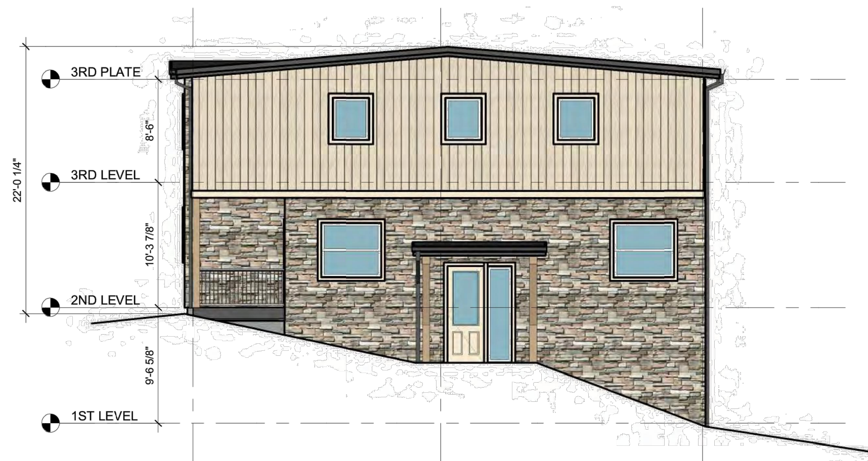
4 5-PLEX - LEFT SIDE ELEVATION 1/8" = 1'-0"
