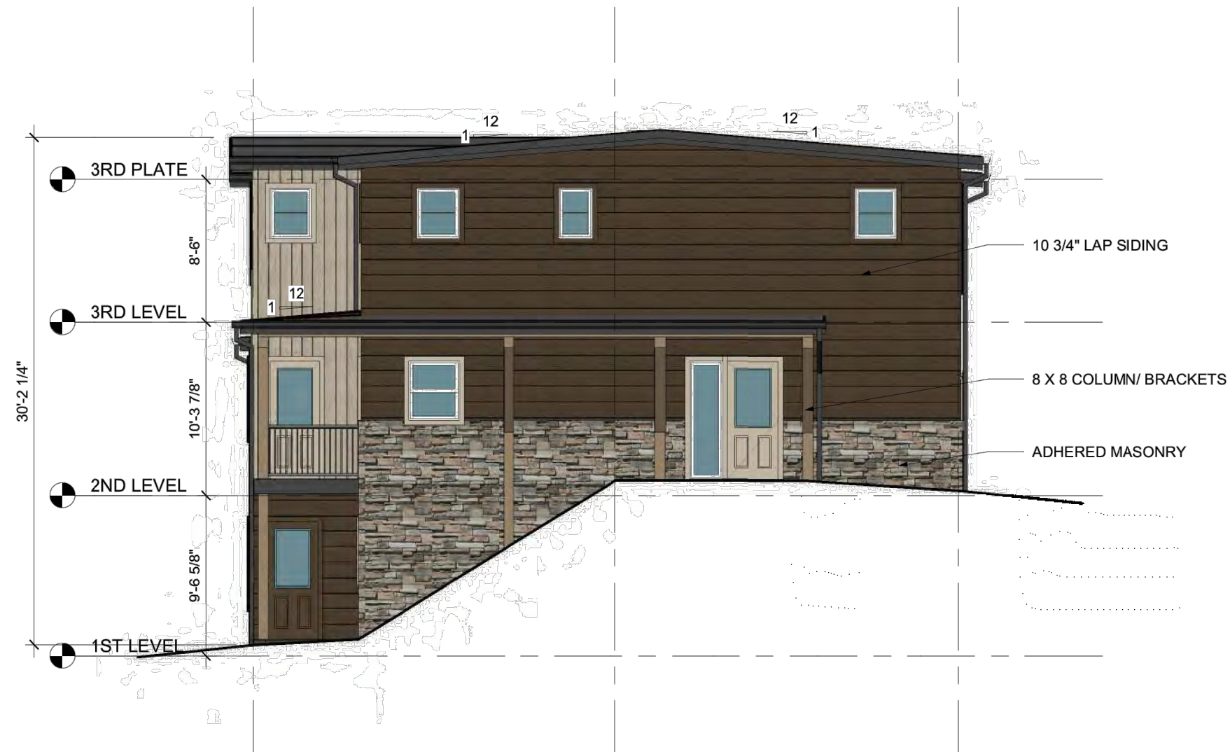
2 7-PLEX - RIGHT SIDE ELEVATION 1/8" = 1'-0"
