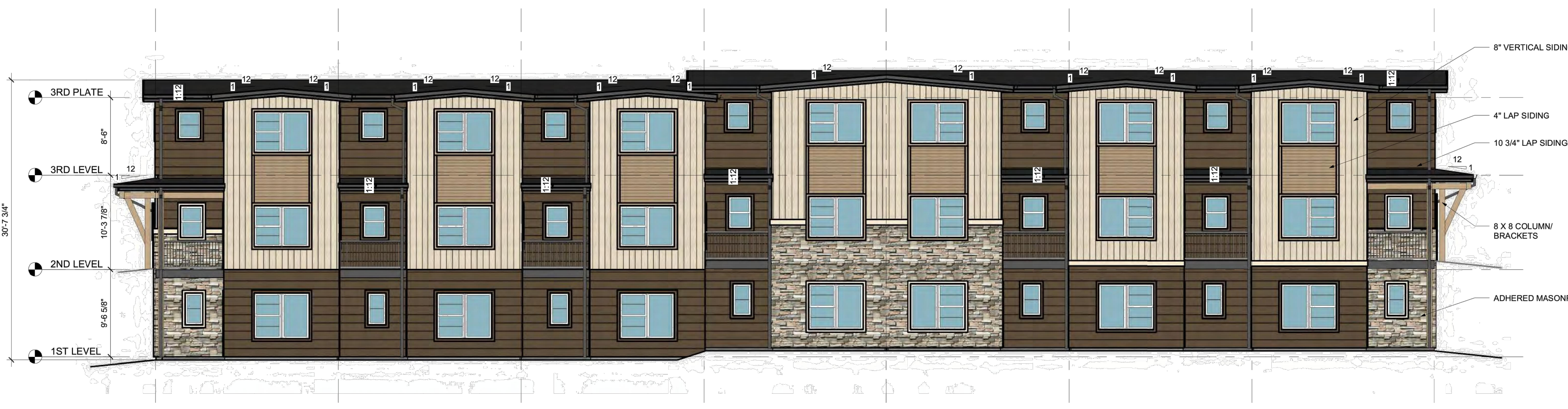
1 7-PLEX - FRONT ELEVATION 1/8" = 1'-0"
