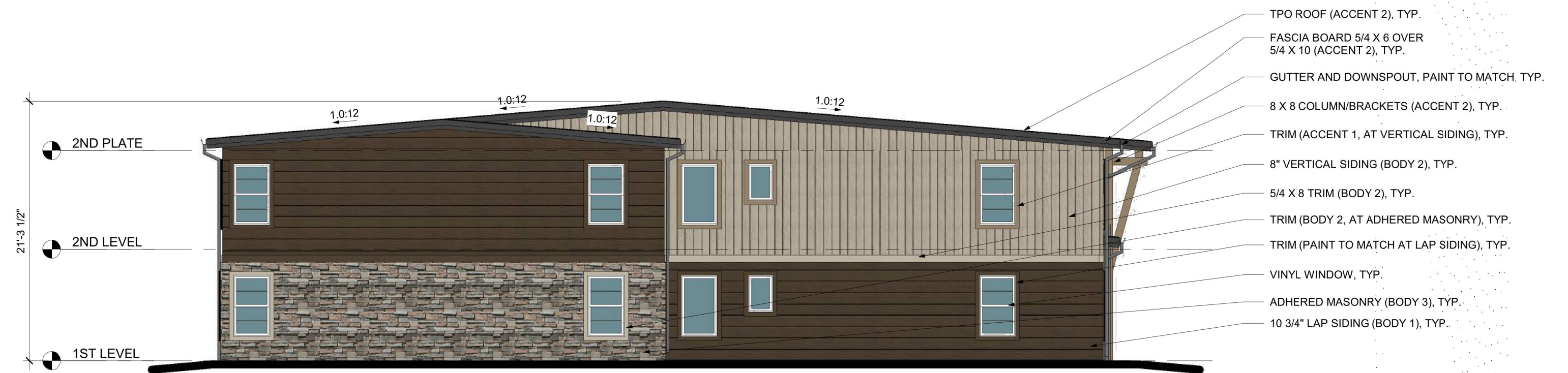
2 BUILDING 3 - SOUTH ELEVATION 1/8" = 1'-0"
