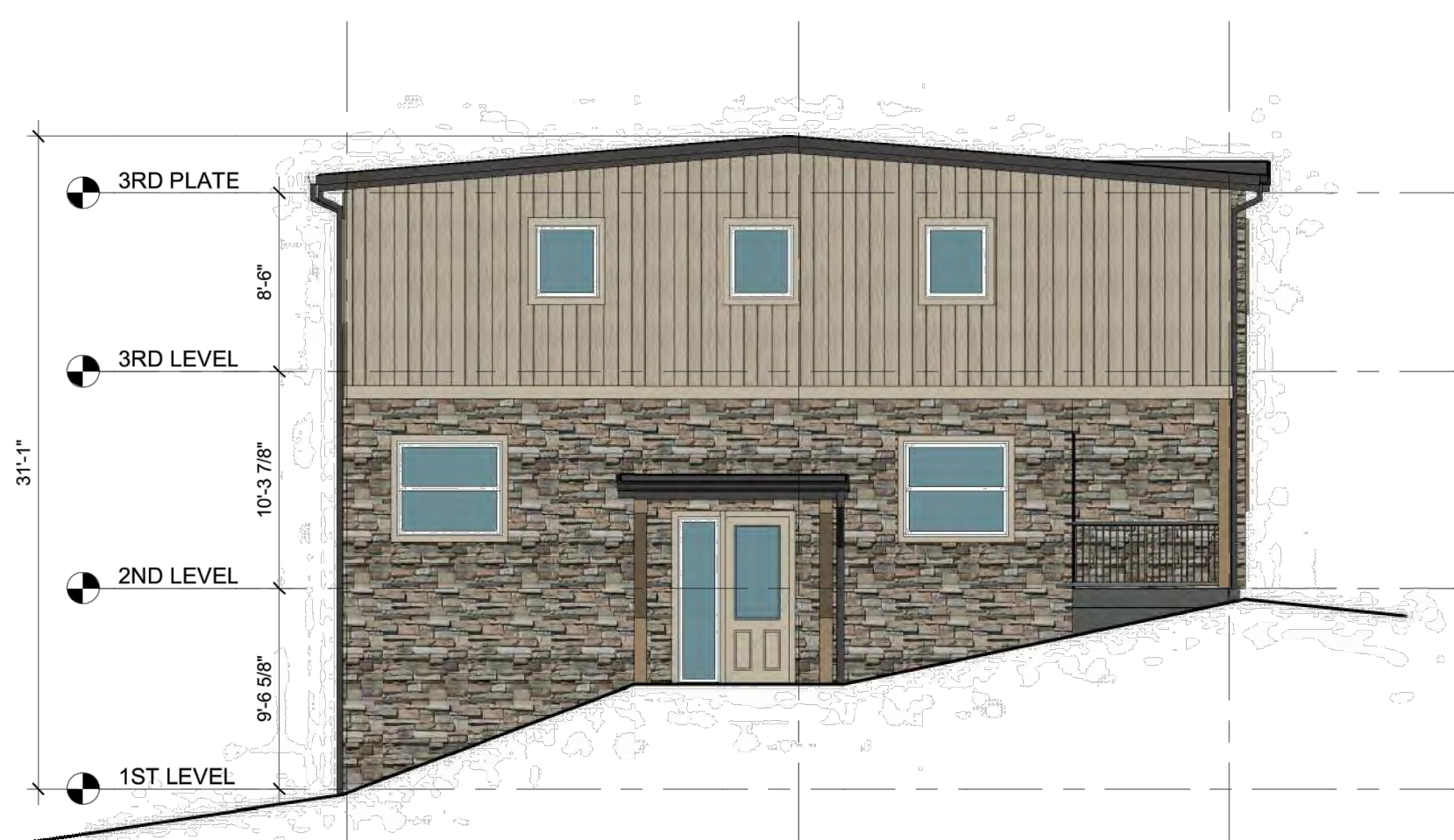
2 5-PLEX - RIGHT SIDE ELEVATION 1/8" = 1'-0"
