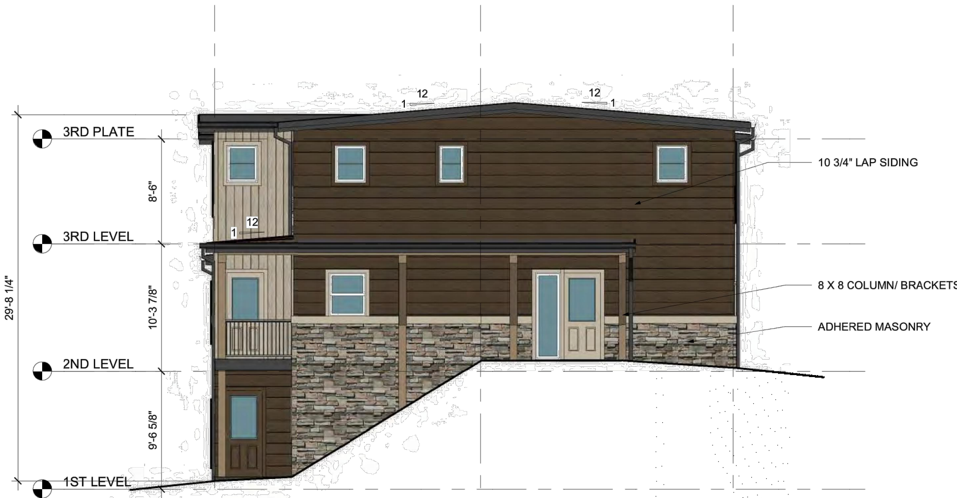
2 4-PLEX - RIGHT SIDE ELEVATION 1/8" = 1'-0"
