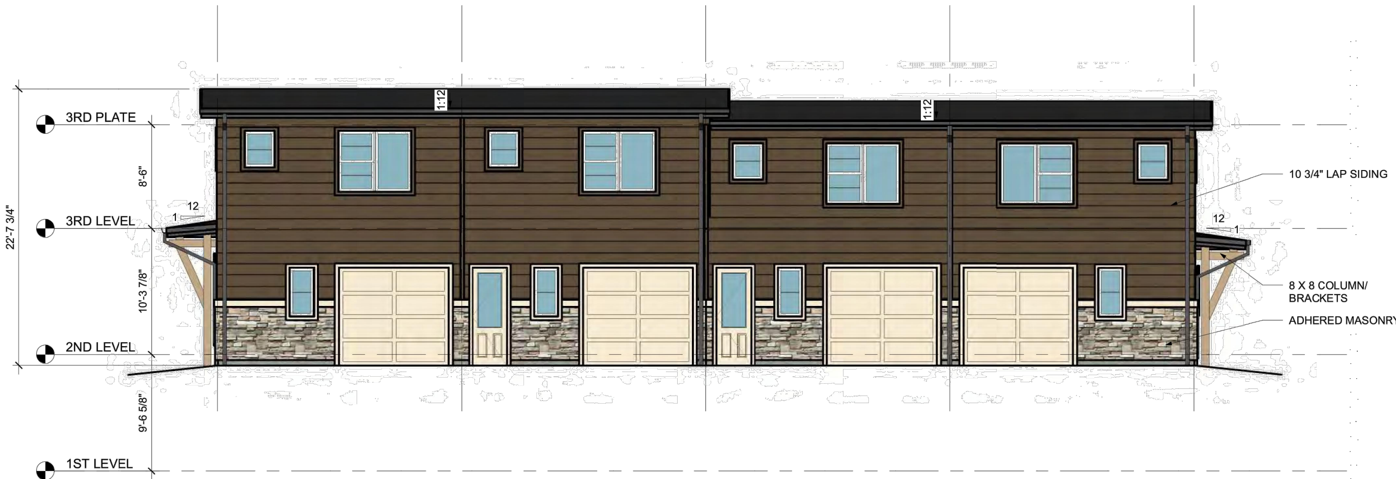
3 4-PLEX - REAR SIDE ELEVATION 1/8" = 1'-0"
