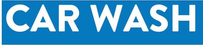
X SIGNAGE ACRYLIC FACE WHITE CHANNEL LETTERS WITH ALUMINIUM RETAINERS CAR WASH 3'-6" x 24'-7"
